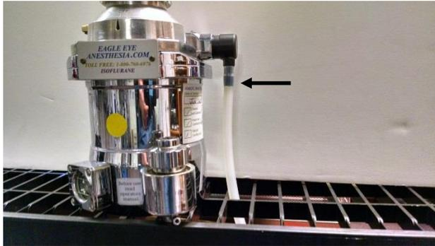
Remove the current opaque silicon hose from the vaporizer outlet adapter which is located on the right (outlet) side of the vaporizer if you are facing the front of the vaporizer.
