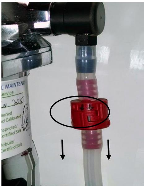
The arrows **MUST** point downward in the direction of gas flow.
