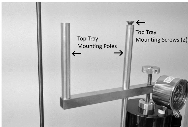
Place both Tray mounting poles into the mounting holes (right and left) and tighten completely (best if done by hand to avoid scratching the brushed aluminum surface). There should now be two mounting poles (Left and Right), one top **right** absorber rod bolt (never removed) in place.
