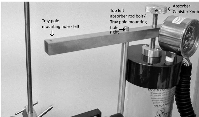
Loosen the **Absorber Canister Knob** and remove the soda sorb canister for this procedure. Using the enclosed 3/16<sup>th</sup> Allen wrench remove the **Top Left Absorber Rod Bolt**. **This bolt can be discarded.** This will reveal the **Tray Pole Mounting Hole-right**.
