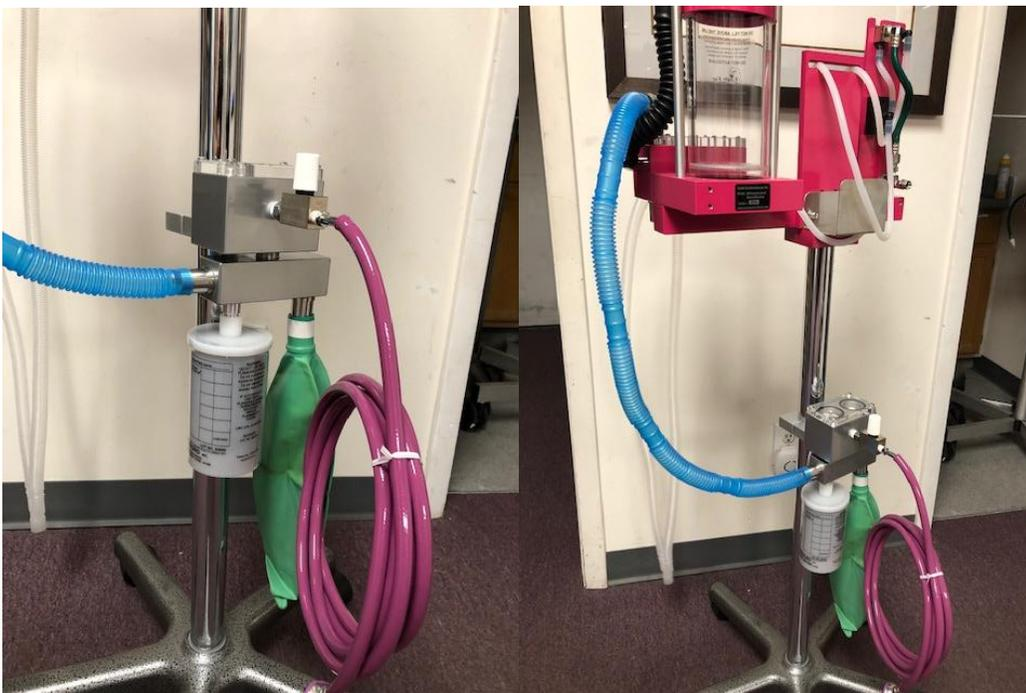
Both chambers are visible through the clear check valve cover to assure proper functioning. The unit mounts directly to the pole of the machine by means of a pole bracket, to a wall by means of a wall bracket or by means of custom bracket/adaptor.
