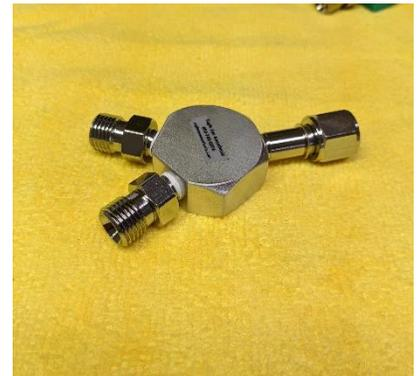
**One-way check valves** – **Never to be used as a splitter.** O2 will not flow out of the male DISS fittings.
