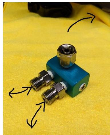
**Open (no valves)** – OK to use with ventilator if the hoses will always stay attached. Otherwise use one with Demand Check valves.
