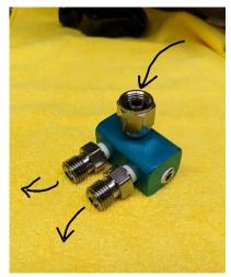
**Open (no valves)** – Only to be used if O2 hoses will not be removed on a routine basis.
