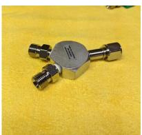
One-way check valves - Never to be used as a splitter. O2 will not flow out of the male DISS fittings.
