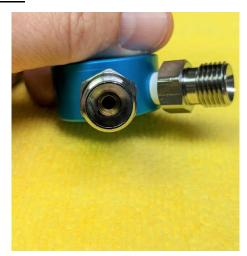
**Demand Check valves** – When hose is attached valve is open and flow can go either way unrestricted. When hose is removed, valve is closed. End of valve extends close to the end of the of male fitting.
